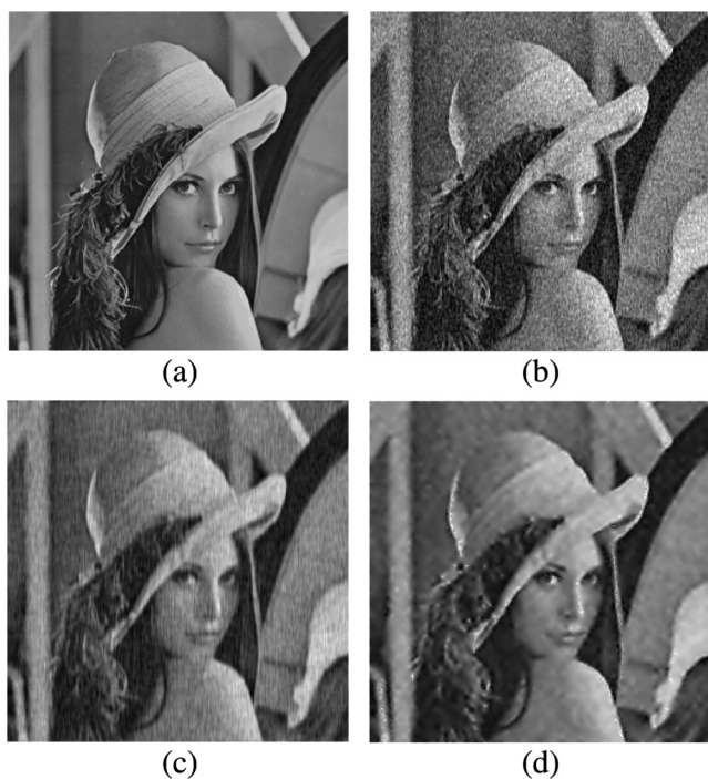
Fig. 4 Comparison of denoising results by using fractional-order Perona and Malik (PM) model and our proposed model on Lena. (a) Original image; (b) Damaged image with \sigma = 25 Gaussian noise (PSNR = 20.1500); (c) fractional-order anisotropic diffusion model (PSNR = 26.4880, \alpha = 1.2 ); (d) Our proposed model (PSNR = 27.4676).
