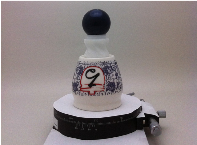
Fig. 22 Photograph of target plastic sphere with black color and high specularity.
