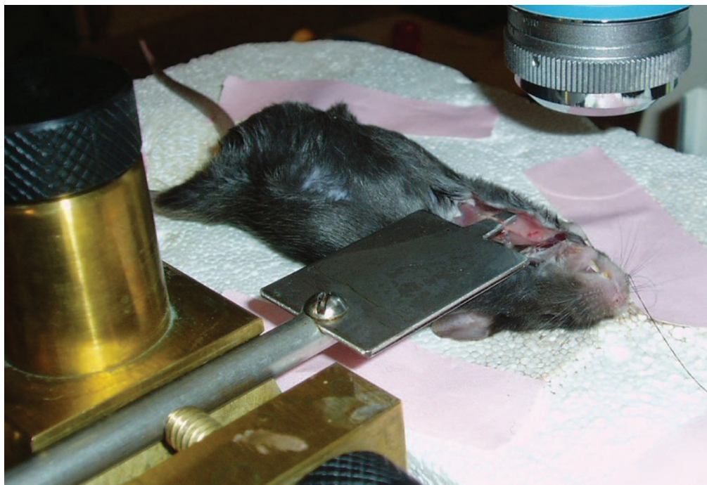
Fig. 1 Prototype of an artery holder and a setup for in vivo imaging of carotid artery.
