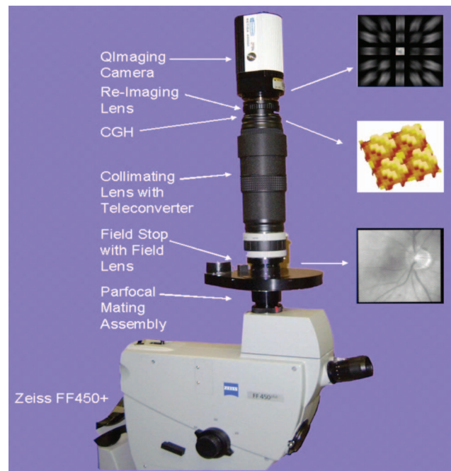
Fig. 2 Zeiss FF450+ fundus camera shown with CTIS attached. The normal 35-mm format image from the Zeiss is field-stopped by the CTIS (insert, bottom right) and relayed using demagnification through the computer-generated holographic (CGH) grating (insert, middle right). Diffraction patterns are shown (insert, top right).
