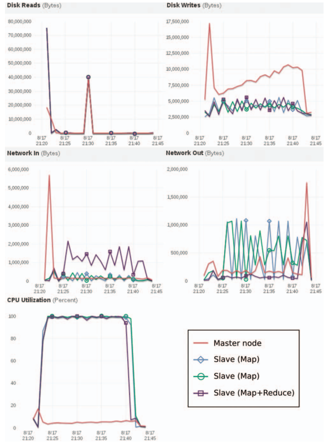
Fig. 7 Resource profile showing I/O and computing during simulation of 300 million photons on a 4-node Hadoop cluster.
