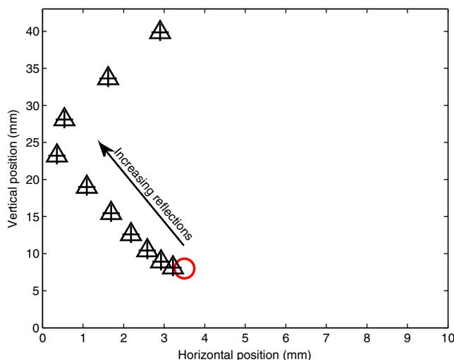
**Fig. 17** Plot of the contributions to the reconstruction for the first 20 reflections where one wall is 1 deg away from perpendicular in a reflective cavity 10 mm long. The circle represents the initial location, the cross and triangles represent contributions from the odd and even reflections, respectively.
