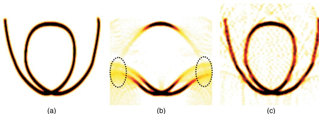
**Fig. 5** (a) Initial pressure distribution, (b) reconstructions without reflections and (c) with reflections are shown. Note that including reflections improves visibility of features that are tending toward perpendicular relative to sensor. Artifacts are highlighted in (b) by dashed lines.
