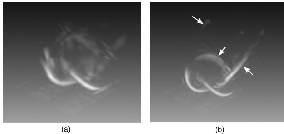
**Fig. 11** Reconstructed initial pressure distribution displayed using Amira. (a) With only a few reflections ( $t_{\max} = 6.8 \mu\text{s}$ ). (b) With all reflections ( $t_{\max} = 22.6 \mu\text{s}$ ). Arrows in (b) highlight regions of improvement in reconstruction using more reflections. Note that the tube on the left-hand side of (b) is at a higher angle relative to the sensor and hence is not reconstructed.
