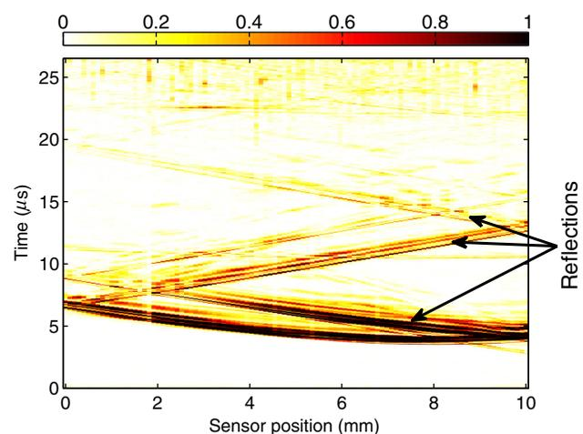
**Fig. 10** Normalized pressure time series experimentally measured using the phantom shown in Fig. 9(b). Note that the reflections can be seen as a series of waves crossing the sensor surface, highlighted with arrows.
