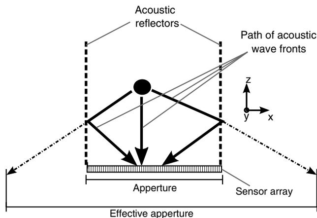
**Fig. 2** Diagram demonstrating the technique developed to extend the effective aperture of a planar sensor array by using acoustic reflectors that are perpendicular to the sensor surface. Here, a side view of the reflector geometry with arrows indicating the effective extension in the aperture due to the reflection is shown. (The effective aperture size will, in general, be different for different points in the image.)
