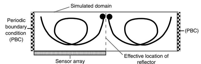
**Fig. 3** Image of the numerical phantom used to simulate the acoustic field when reflections are present. Note the mirrored copy on the right-hand side (the circles at the tip of the phantoms are not present in the simulation and are shown here to illustrate the mirroring).
