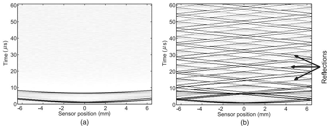
**Fig. 4** The first  $60 \mu\text{s}$  of the pressure time series from simulation, (a) with no reflectors present (b) with reflectors present. Time series were recorded up to  $380 \mu\text{s}$ , but this first  $60 \mu\text{s}$  only is shown here for clarity. The arrows draw attention to the presence of reflections in (b).
