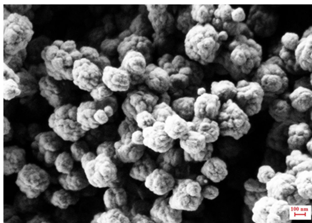
Fig. 10 SEM image of the \text{NaY}_{0.8}\text{Yb}_{0.17}\text{Er}_{0.03}\text{F}_4 nanoparticles sample.
