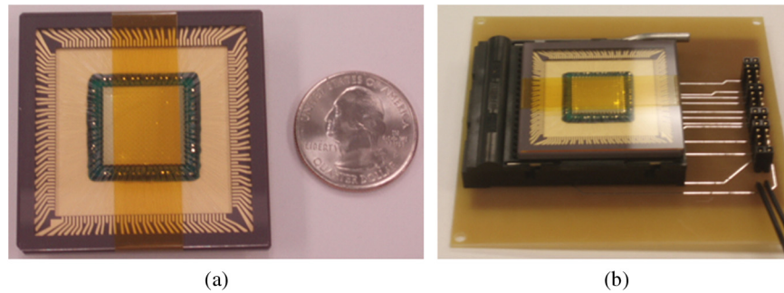
Fig. 4 (a) Top view of the packaged 16 \times 16 array DM. (b) Assembled DM on a PCB test board.
