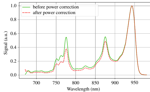
Fig. 9 Signal of one channel as a function of wavelength before (solid) and after (dashed) power correction.
