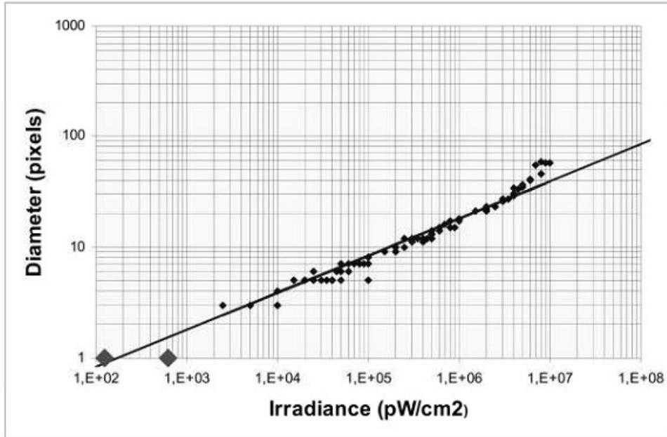
Figure 8 Spot size vs. laser power
