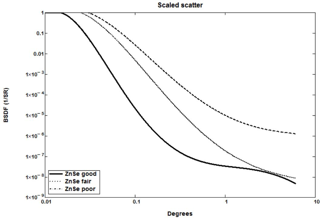
Figure 4 Bi-directional Scatter Distribution Function
