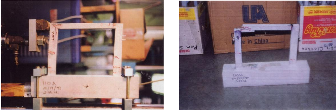
Figure 2) Photo of frame containing internal self-repairing adhesives, cracking in the third static test, which shows cracking all over, but no catastrophic failure [4]
