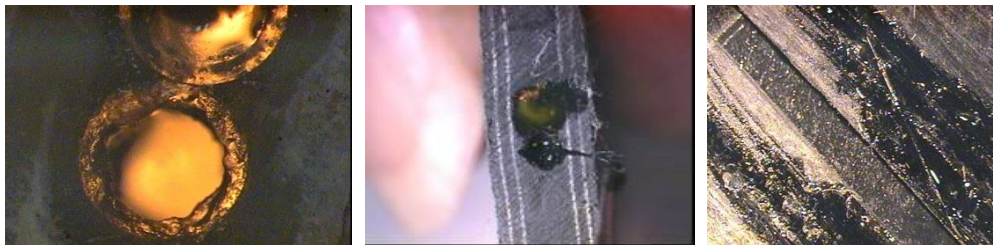
Figure 9) Left, repair chemicals survive heating in graphite laminates at 350F for two hours after one hour at 250°F. Middle, cut glass repair fibers after processing in the autoclave exhibiting liquid inside and Right, a cut through sample showing that the repair chemical filled an area of delamination.
