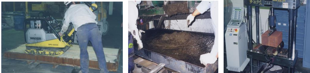
Figure 15) Left two, manufacturing fly ash panels at a company, Right, Testing fly ash bricks
