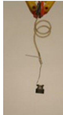
Figure 16: Shape memory programmable and electrically controllable IPMC
