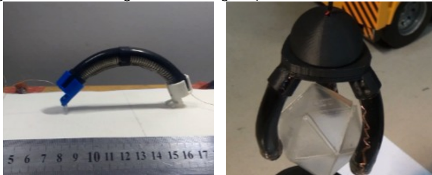
Figure 5: Soft robot and soft gripping device based on DE Actuators
