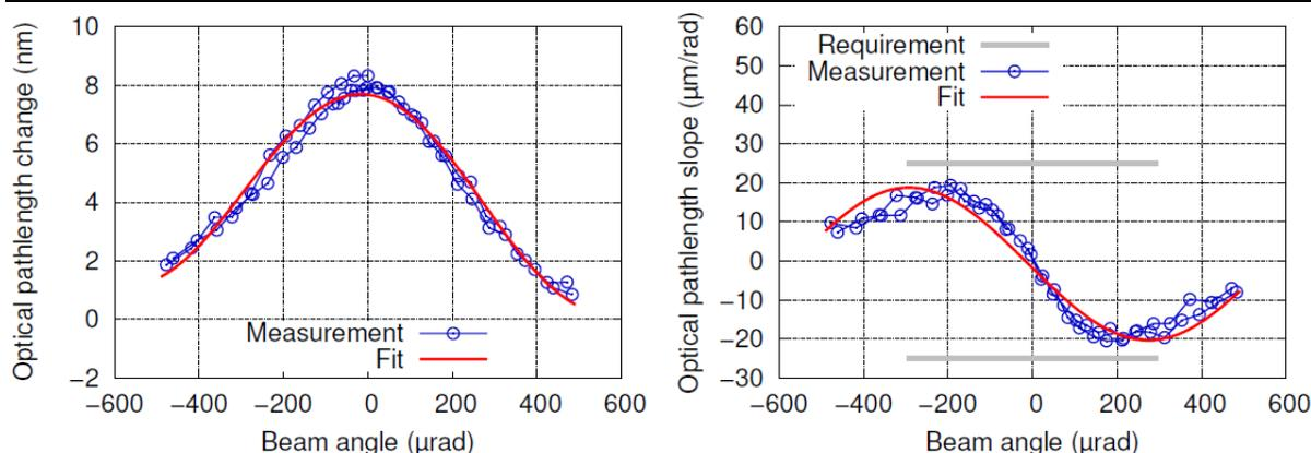
**Fig. 7** Two-lens imaging system: nominal performance with Gaussian RX beam and 1m focal length lens in front of RX FIOS on telescope simulator. Left: Path length change vs. beam angle, right: Slope of path length change vs. beam angle.
