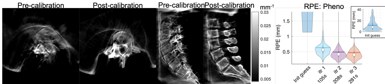
Figure 7. Experiment C - Artis Pheno: (Left) selected axial and sagittal slices from pre- and post-calibration reconstructions of torso phantom. Voxel size: 0.5 x 0.5 x 0.5 mm. (Right) Summary of RPE as a function of iteration.
