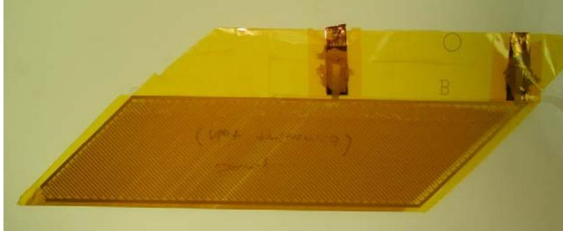
Figure 3. The Active Fiber Composite Actuator.
