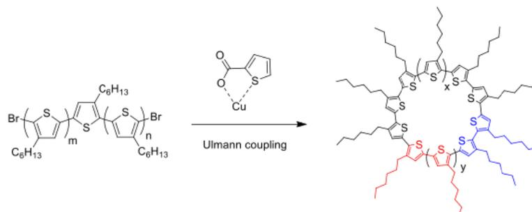
A very difficult problem in the synthesis is the strong competition with interchain coupling requiring synthesis at (extremely) high dilution. Moreover the separation of the macrocycles from linear polymers – both having comparable chemical properties – is as yet an unresolved issue.
