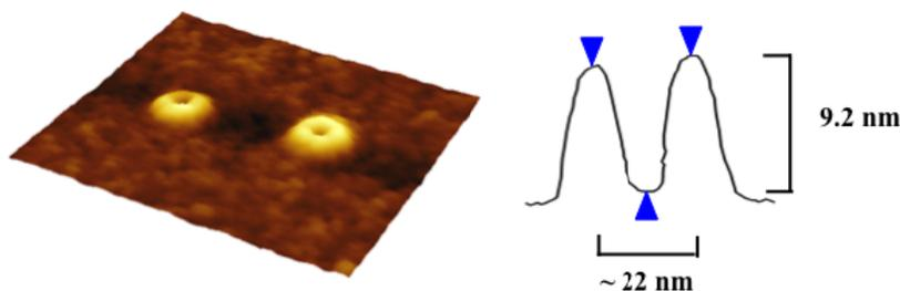
Fig. 3 AFM picture of a film showing the presence of doughnut structures in films of poly(3-dodecylthiophene).
