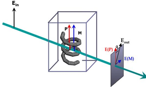
Fig. 1 The interaction of an optical field with a chiral structure, electric dipole and magnetic dipole radiation result in rotation of polarization.
