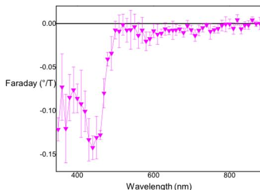
Fig. 4 Faraday rotation measured in a chloroform solution 0.7 mg/ml of the “Coulembier” macrocycle; sample cell thickness 1 mm
