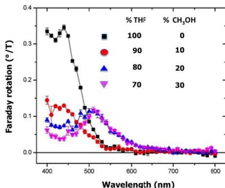
Fig. 2. Faraday rotation in solutions of poly(3-octylthiophene) in different solvent compositions at a concentration of 0.25 mg/ml, sample cell of 1 mm thickness
