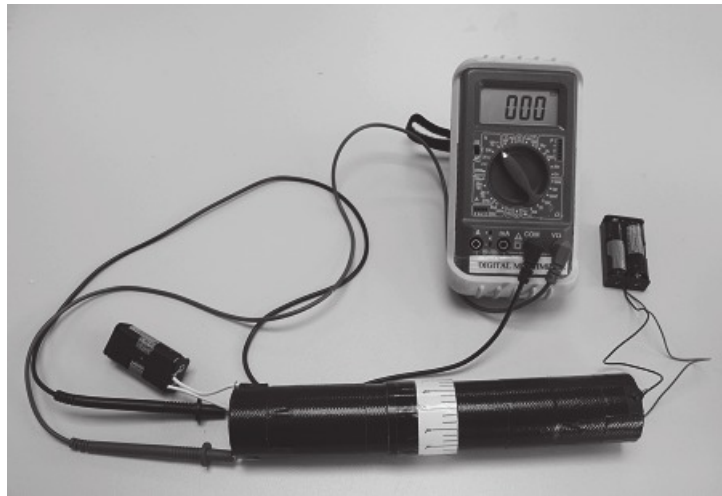
Figure 9: Set up of models to verify Malus's Law quantitatively.
