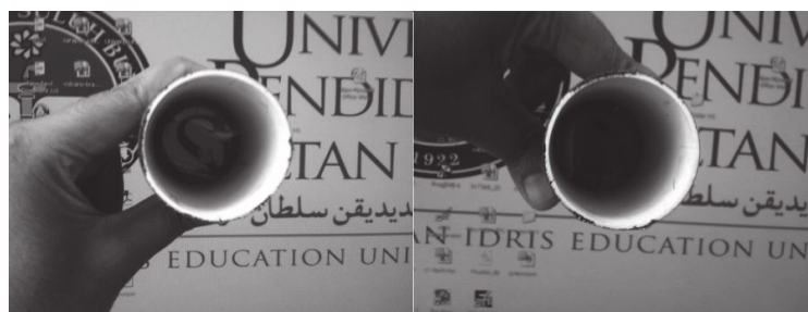
Figure 7: Determining the polarization direction of the polarizer. Left: The direction of light polarization is parallel to the polarizer. Right : The direction of light polarization is perpendicular to the polarizer, therefore the emitted light is blocked (dark).
