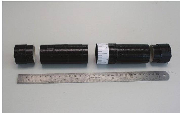
Figure 3: The assembled and ready polarizer tube made from raw materials in the Figure 3.
