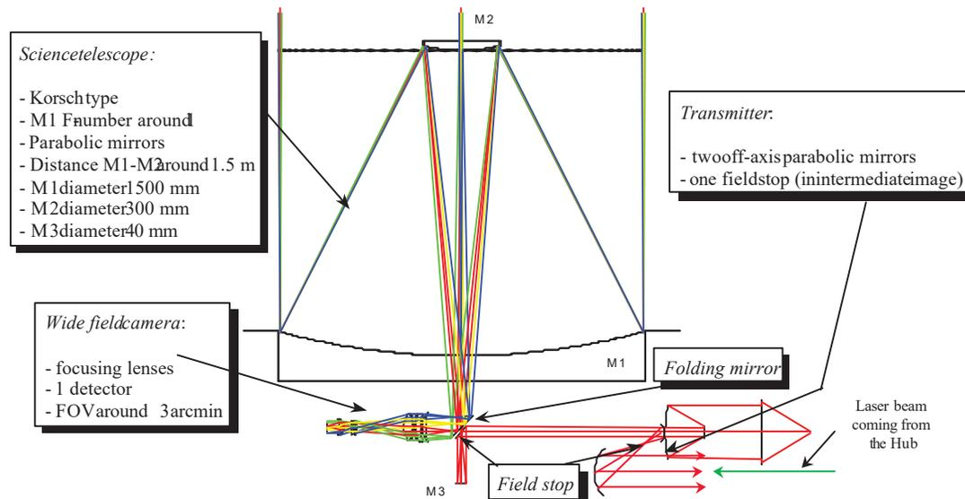
Figure 3 Telescope collector optical concept
