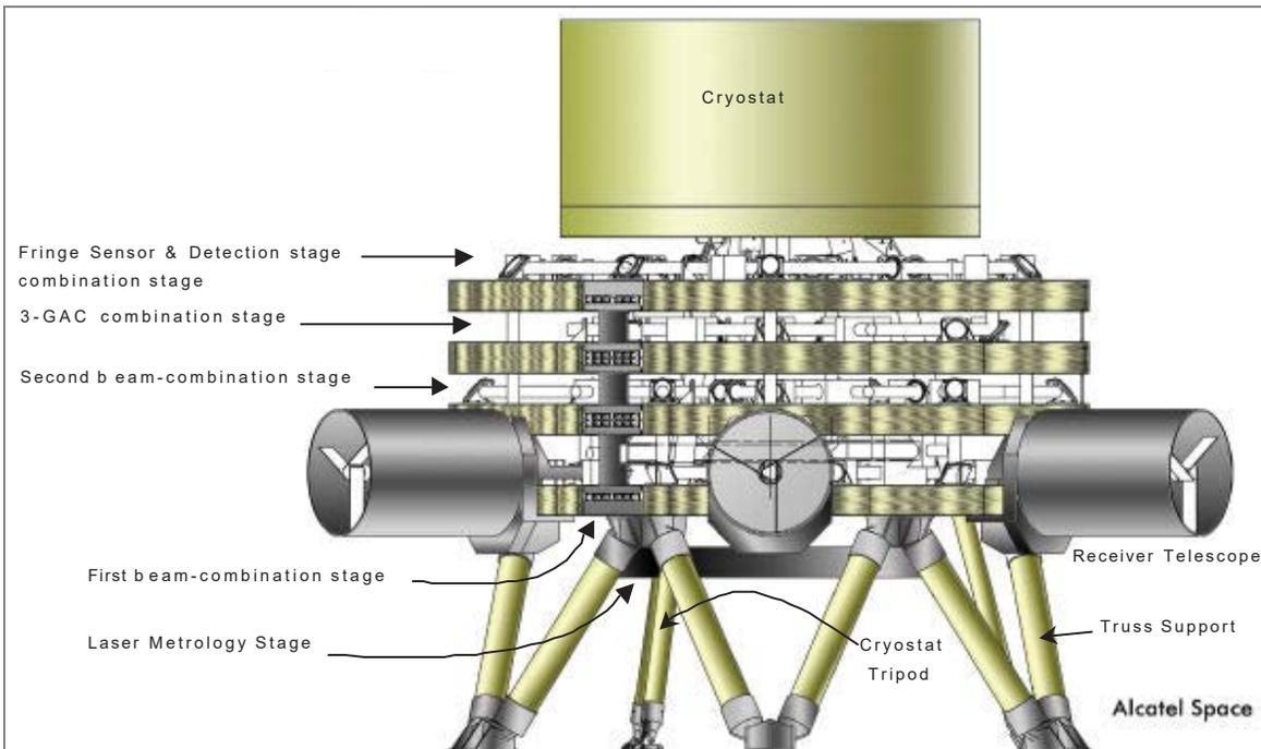
Figure 11 Beam-combiner mechanical architecture
