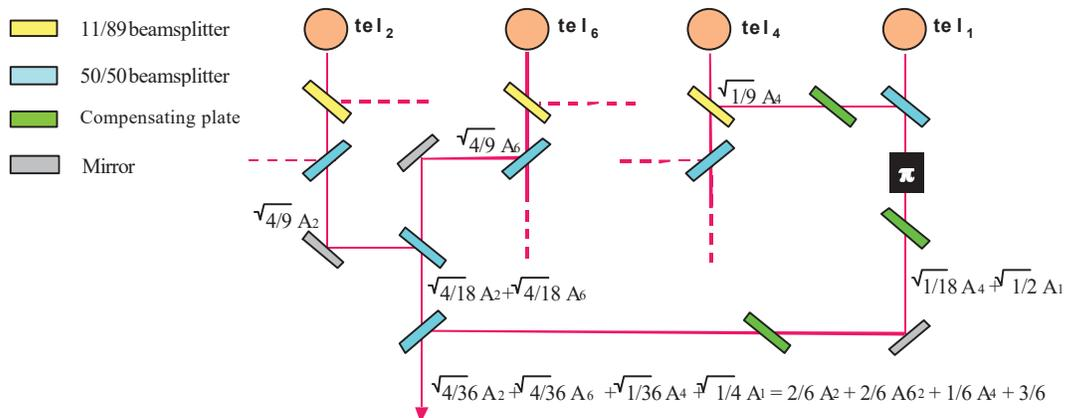
**Figure 5** Beam-combining principle of the 3-GAC nulling interferometer
