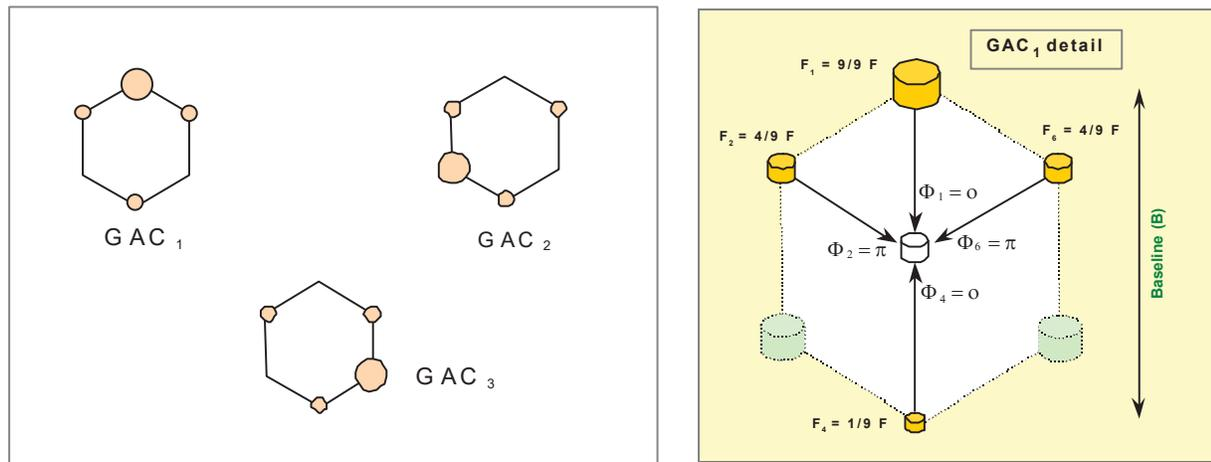
**Figure 1** The Laurance nulling space interferometer consists of 6 equal size telescopes flying in a hexagonal formation, with the beam-combiner in the centre.
