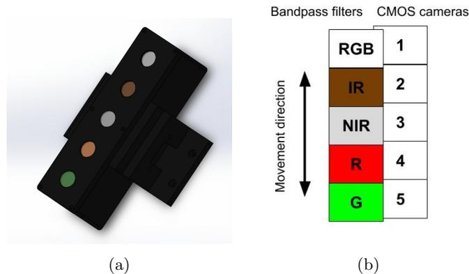
Figure 3: Multispectral camera system developed for acquisition of multispectral images of weeds and soybean plants. (a) Tridimensional concept; (b) bandpass filters array.
