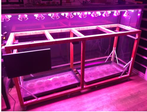
Figure 2: Automated v-slot rail system developed to automate image acquisition and to simulate the movement of a spray tractor in the field towards crop's planting rows.
