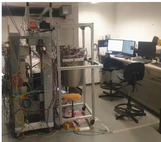
Figure 2: Picture of the physics package of the flight payload of the MAIUS-2 sounding rocket mission serving for functional tests performed with test hardware of lasers and electronics. The physics package is covered by a three-layered cylindrical magnetic shield.
