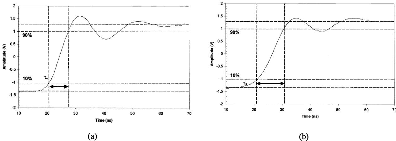
Figure3: Rise time of (a) the laser / receiver system, and (b) the laser, the 3.46km fiber link and the receiver.
