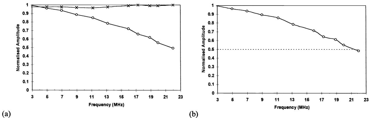
Figure 4: (a) The measured frequency response of the transmitter/receiver {o} and of the full optical system with 3.46km of optical fiber {x} and (b) the optical fiber frequency response calculated from the other two
