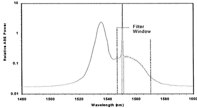
Figure 8: Relative variation of ASE power with wavelength from the EDFA showing the fraction of power in a  $1\text{nm}$  band (shaded region) around the signal wavelength.
