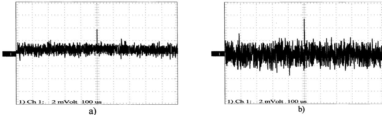
Figure 6: ASE-ASE beat noise for incident ASE powers of  $-4.0\text{dBm}$  and  $-7.0\text{dB}$ .
