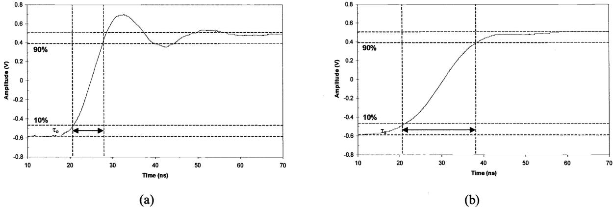
Figure 2. Rise time of (a) LED / receiver system, and (b) LED, 2.23km fiber reel and receiver system
