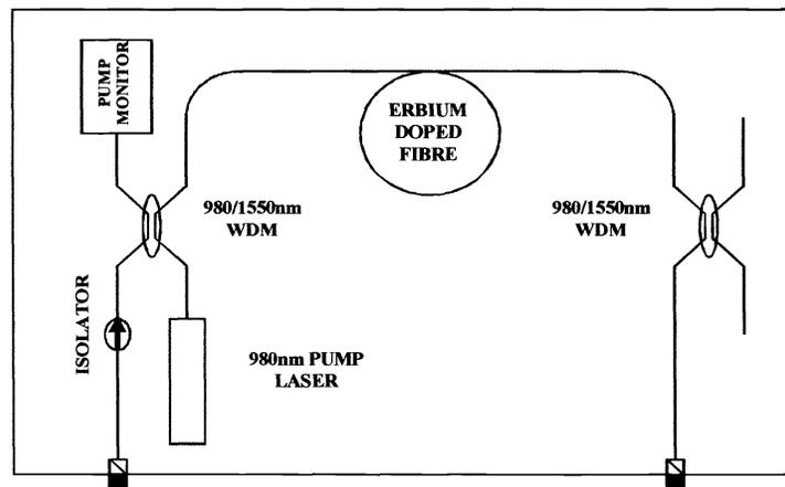
Figure 5: Schematic diagram of EDFA
