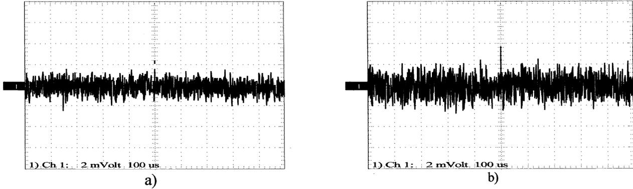
Figure 7: Signal-ASE beat noise for incident signal power of a)  $-8.5\text{dBm}$  and b)  $-2.5\text{dBm}$  and ASE noise power of  $-10\text{dBm}$
