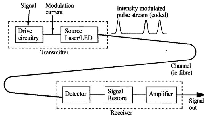
Figure 1: Schematic of a point to point fiber optic communications link.
