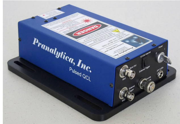
Fig. 12. An tabletop version of uncooled (no TEC) QCL package that produces > 2\text{ W} at 4.6 \mu\text{m} and > 1.5\text{ W} at 4.0 \mu\text{m} and operates from a standard 12-24V DC computer grade power supply.
