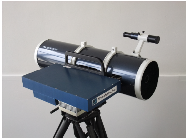
Fig. 19. Multiple tunable QCL and light collection system for standoff detection of trace explosives residue.
