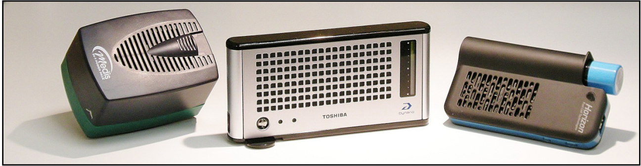
Figure 5: Images of commercially purchased fuel cells designed for portable electronics Left to right: Medis 24-7 Power Pack, Toshiba Dynario, and Horizon MiniPAK.
