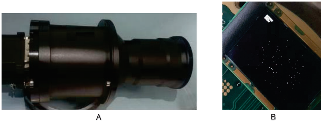
Figure 2. The MINISTAR: (A) the assembled prototype, and (B) a detail of the monitor with the rendered star field.
