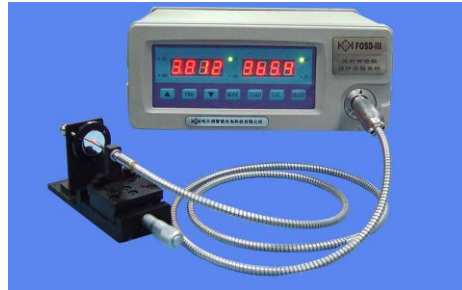
Figure 1 The fibre-optic sensor with intensity compensation model
