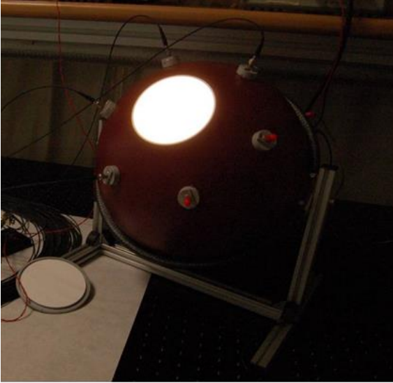
Fig. 18 the 300 mm integrating sphere for fast verification procedures
