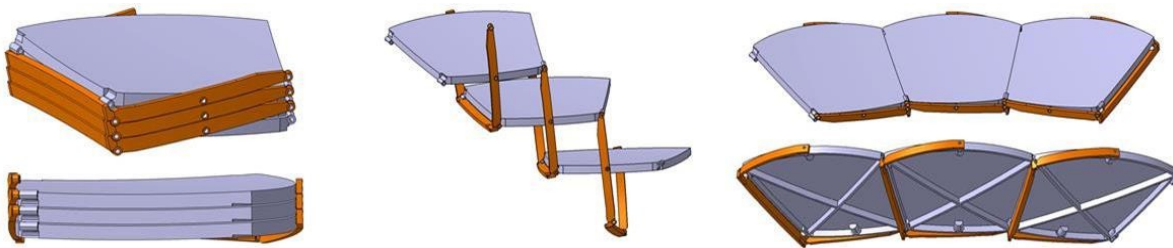
Fig. 5. Deployment of subset of segments of TALC to be tested in cryogenic conditions
