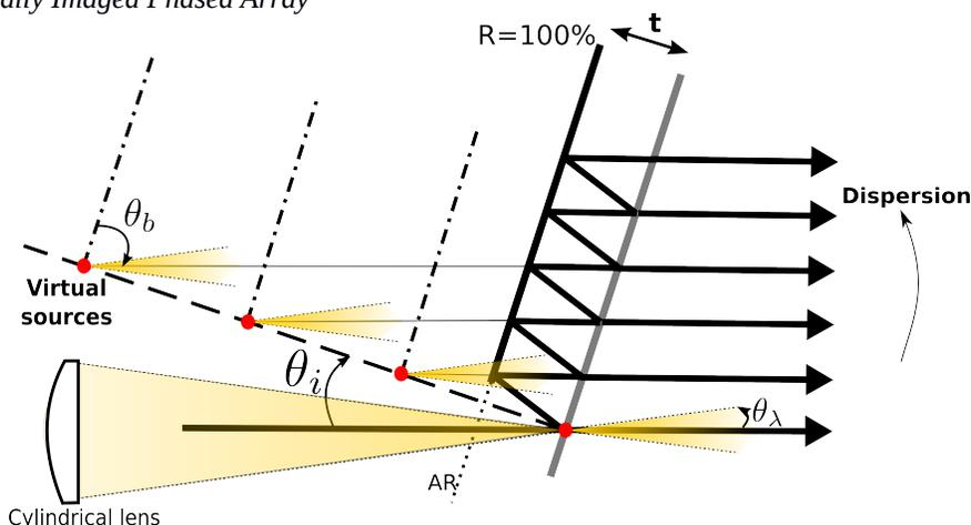
**Fig. 1.** : VIPA geometry, showing the multiple bouncing on the reflective plate and the equivalent virtual sources
