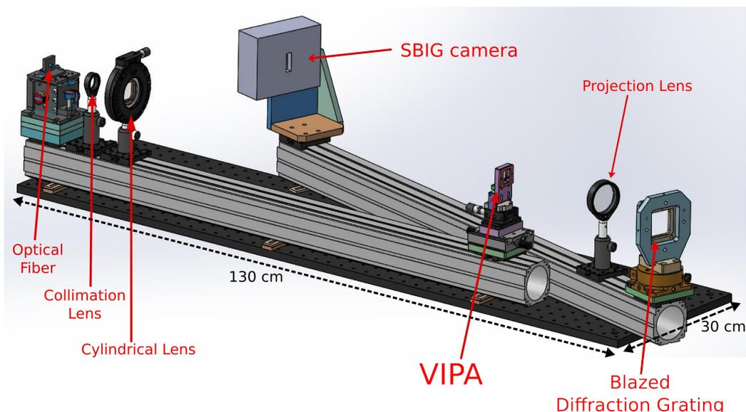
Fig. 3 : Model of the demonstrator intended to achieve  $R= 570\ 000$
