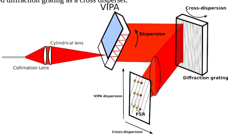
**Fig. 2 :** Principle of an échelle-spectrometer based on the VIPA. The optical design is analog to that based on a classical échelle-grating.
