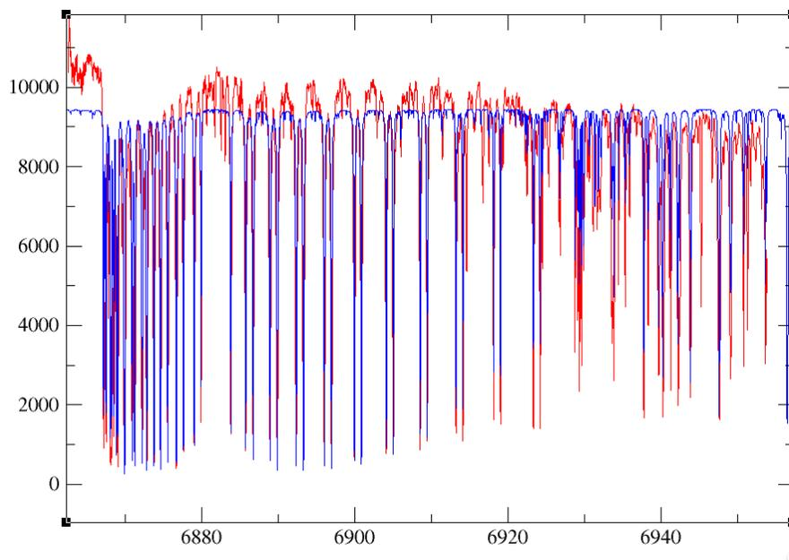
**Fig. 5** : Complete wavelength range of the spectrum of the sun observed with the VIPA, and its comparison with a simulated spectrum of the telluric lines above our observation site, provided by the SkyCalc Sky Model Calculator (ESO).
