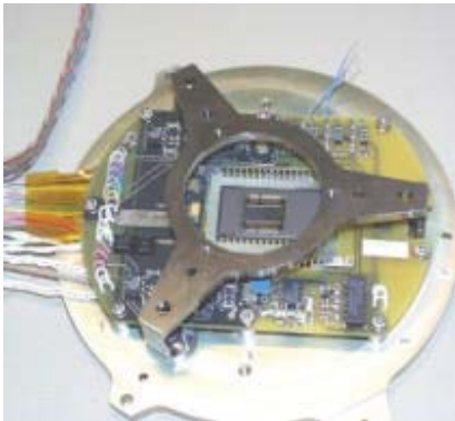
Figure 4: View of micro-sensor optical head
