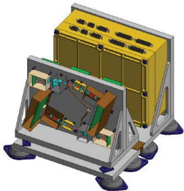
Figure 3: The architecture of the AOS (preliminary design)
