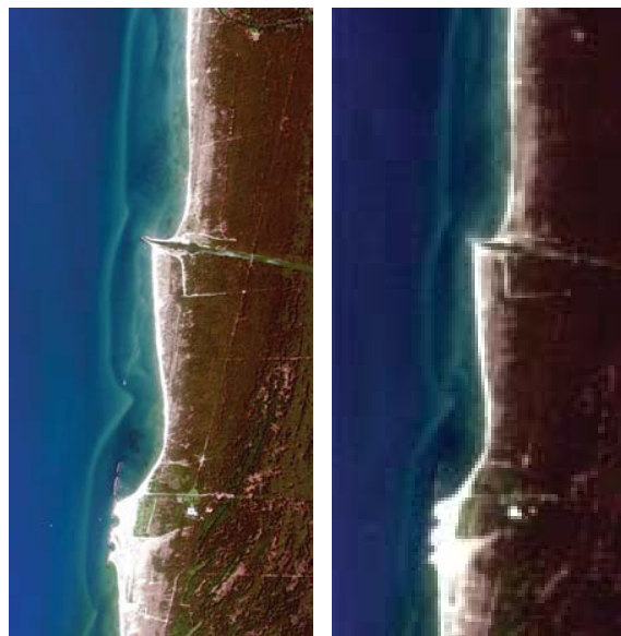
Fig.3: a) RGB of the input MIVIS airborne reflectance image (2.5m); b) RGB of the output simulated Radiance (20 m)
