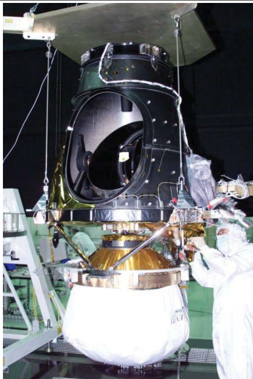
SEVIRI Instrument Main Unit during integration, showing the TSA cone aperture
