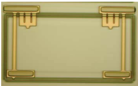
Fig. 2: Optical microscope image of the backside a microfabricated single mirror of a micromirror array. The 100 \times 200 \mu\text{m}^2 mirror is suspended by two cantilever flex-hinges. The extra pads at the top will be used for the electrostatic clamping mechanism.
