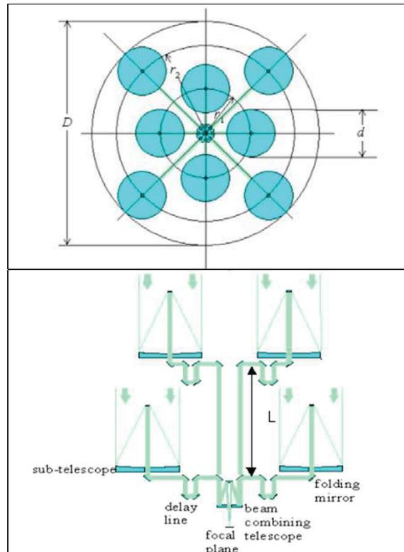
Fig. 5: sub-apertures configuration and interferometer optical concept
