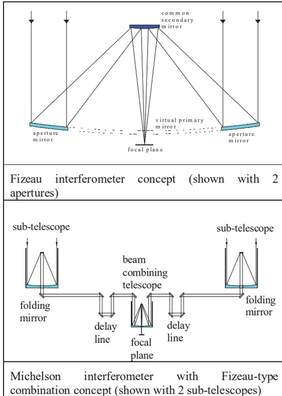
Fizeau interferometer concept (shown with 2 apertures)
