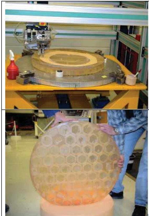
Fig. 11: mirror breadboard in some manufacturing steps
