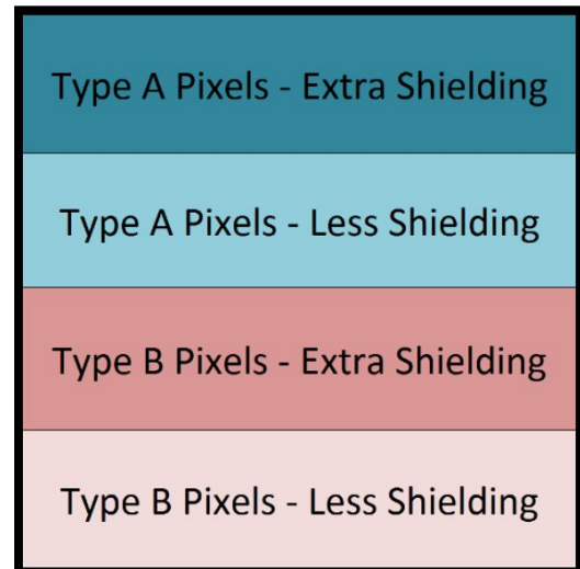
Figure 2. Pixel layout of the small pixel HCD test devices. Type A pixel have no in-pixel CDS while type B pixels do include in-pixel CDS.
