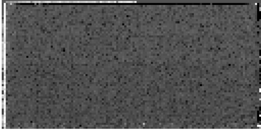
Figure 9. Gain variation map for FPA 18568. Brightness of pixels corresponds to the gain measured in a pixel. The measured gain variation (excluding inactive pixels — many seen at array edges) is 1.23\% \pm 0.1\% .
