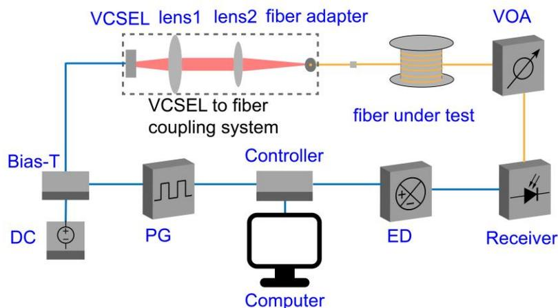
Figure 5. Schematic of the experimental setup for system transmission test. PG: pattern generator; VOA: variable optical attenuator; ED: error detector.
