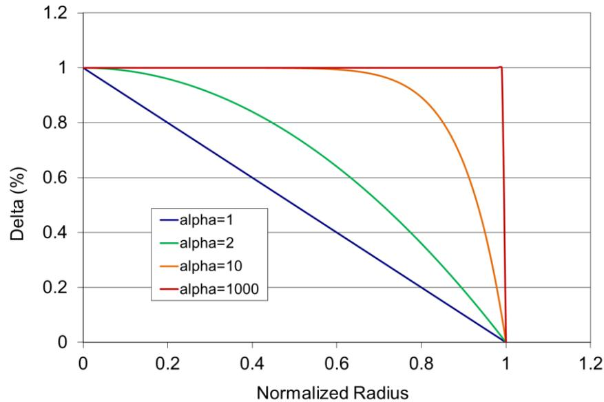
Figure 2. Alpha profiles with different alpha values
