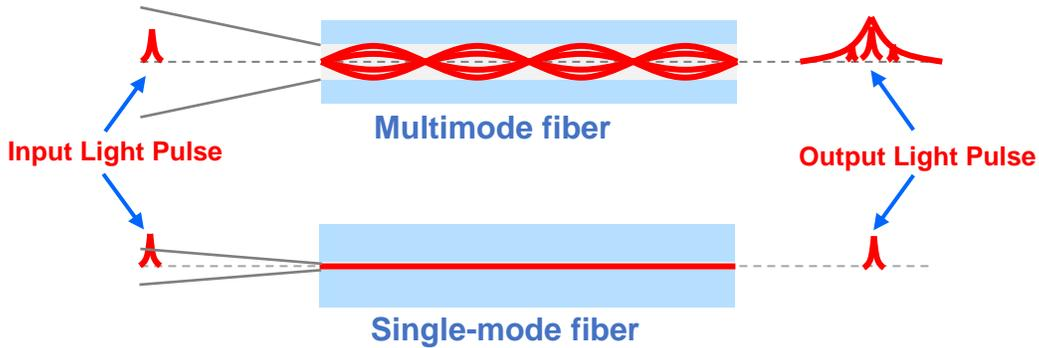
Figure 1. Comparison between multimode and single-mode fibers.
