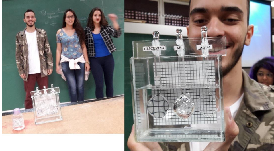
Figure 18. Group of students who did a refraction demonstration using fluids with different refractive indexes: glycerin, air, water ( GLICERINA, AR, ÁGUA ). They showed that the divergent and convergent lens effect also depends on the relationship between the refractive indexes of the lens and the medium.
