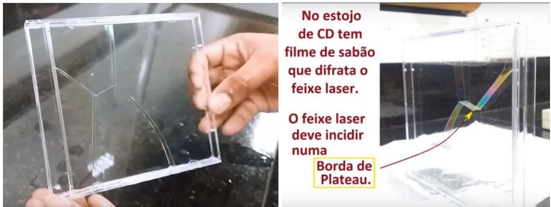
Figure 11. The CD case has soap films that diffracts the laser beam ( No estojo de CD tem filme de sabão que difrata o feixe laser ). The laser beam must reach a Plateau Border . ( O feixe laser deve incidir numa Borda de Plateau ). The Plateau borders are formed in the encounter of liquid films of soap solutions. In these images we can see two Plateau borders that can be used in the experiment. To get these films, we plunged the opened acrylic box into the detergent solution, closed the box and took it out slowly, letting the solution run, more details in the video “Make a HALO with LASER” 29 .
