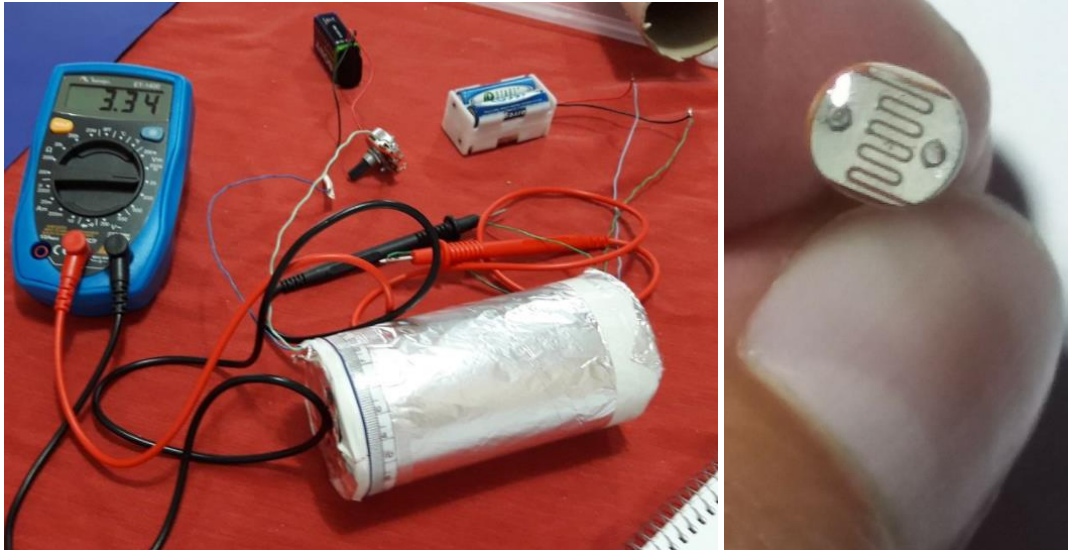
Figure 17. Device constructed according to the work of Kadri, Wei, and Jaafar 5 for study Malus Law. Close-up of the light detector, a LDR, photoconductive cell made of CdS.
