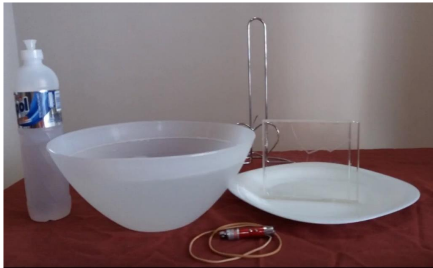
Figure 12. Objects found in the house that can be used for observation of the parlaseric circle. CD case (narrow acrylic box), laser pointer, a tall and thin object used as a pointer holder and aqueous detergent solution.
