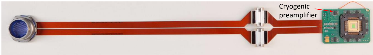
Figure 3 : Detector board with flex cable, two 72-pin Micro-D connectors for penetrating the radiation shield and the 128 pin HIREL vacuum connector.
