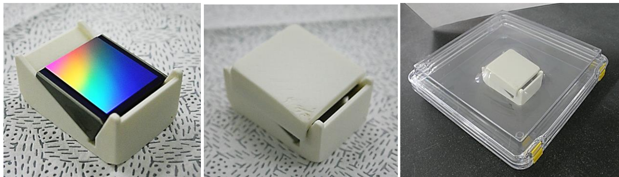
Figure 9. Ge GRISM after AR coating (Left), with protected cover (center) and in the package for transportation (Right)
