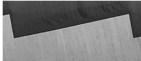
Figure 2. The typical cross section of groove by cutting
