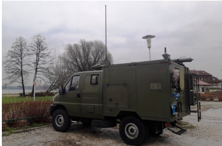
Figure 4. Mobile sensor on the heavy-terrain vehicle.
