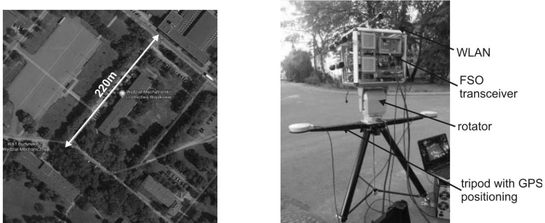
Figure 4. View of the test conditions and the FSO transceiver with GPS positioning system.
