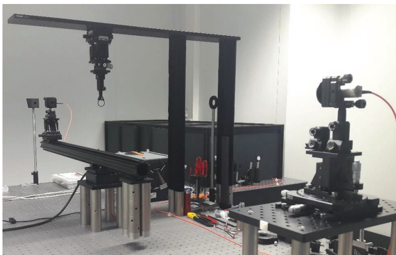
Figure 2 SALSA instrument in ISO6 clean room in the Espace Photonique of Institut Fresnel. Measurement subassembly: a reflective collimator (right) outputs the optical beam which illuminates the sample (middle), the scattered light is collected by a second reflective collimator mounted on a rotating arm (left).
