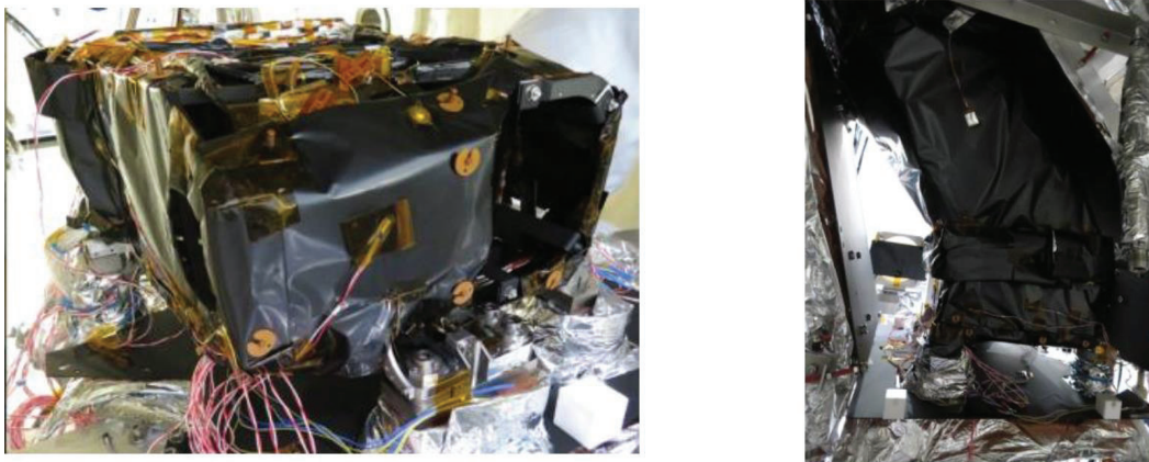
Figure 12. BTA in the thermal tent (only lower shroud is shown). Left – without MLI tunnel. Bottom – with MLI tunnel
