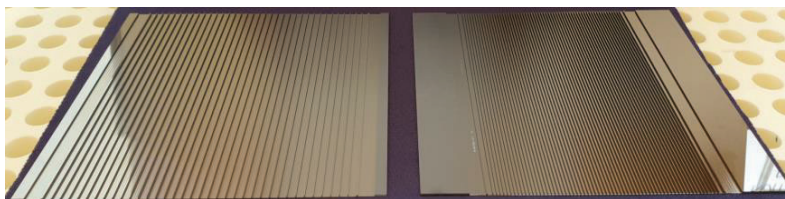
Figure 6: First prototypes of ‘row 08’ mirror plates (left). The increased rib spacing of 2.3 mm is clearly visible, when compared to existing 1 mm rib pitch plates (right).
