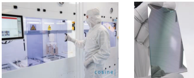
Figure 7: The newly installed fully automated cosine wetbench (left), which includes also an automated lift-off batch for post coating resist removal. The right photo shows a fully processed plate after lift-off, which was taken during the commissioning of the system in Nov 2020.
