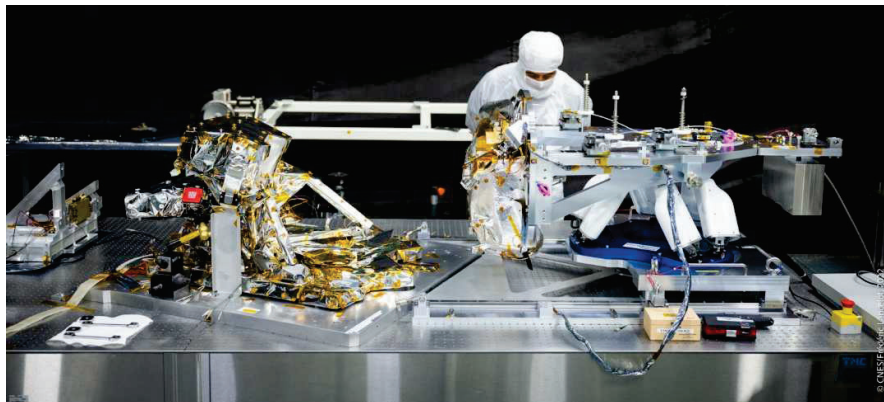
Figure 7. The PCS with the telescope (left) and the spectrometer (right) before the coupling
