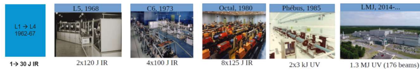
Figure 1: Main generation of high energy, high power laser in operation at CEA from 1962 to 2024. LMJ laser is represented at first light (one bundle = 8 beamlines in 2014) and in its 2024 configuration (11 bundles = 88 beamlines)
