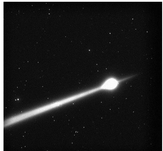
Figure 5 White-light supercontinuum propagating vertically in the atmosphere. White dots are stars in the background.
