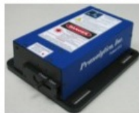
Figure 15. Fully packaged QCL systems for various applications. Note that the OEM QCL butterfly package and the OEM QCL platform meet MIL-STD vibration/shock & temperature requirements (Test protocols derived from MIL-STD-810G).
