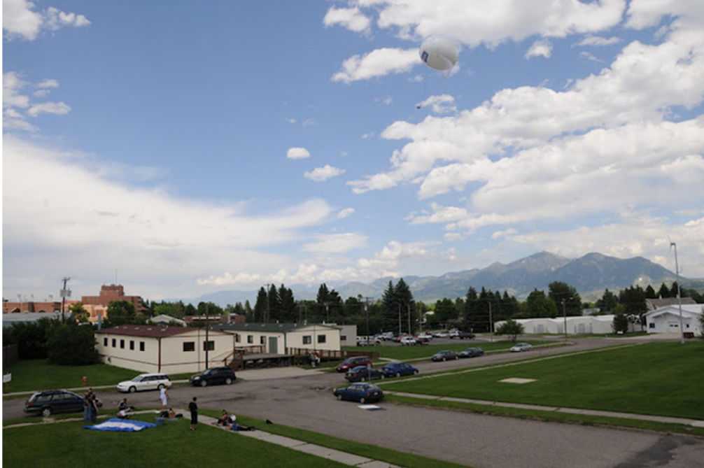
Figure 7. Photograph of tethered balloon carrying multispectral imager during test flight at Montana State University. The tethered balloon is located just right of the upper center, while the calibration panel is at the bottom center, next to a parked car.
