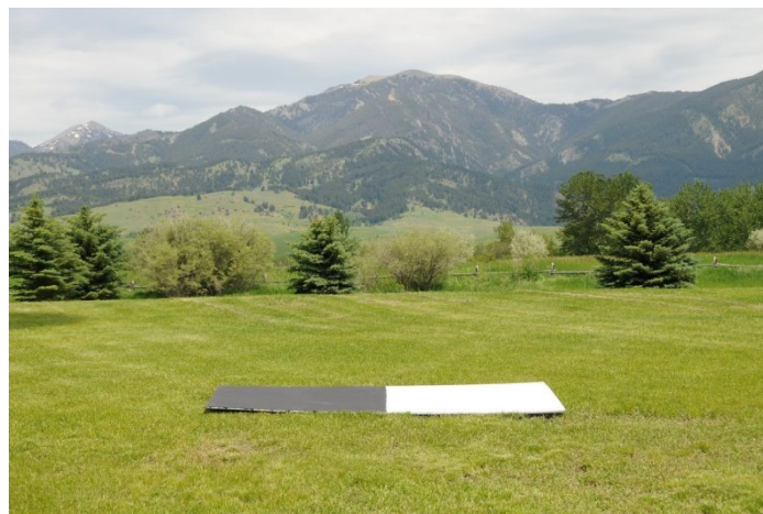
Figure 6. Photograph of a plywood black-and-white reflectance calibration panel, which is laid on the ground within the imager's field of view to provide a reflectance calibration. Later versions were painted on canvas tarps.
