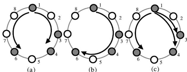
Fig. 2 Example of light trees: (a) SPT, (b) MST, and (c) multicasting in WDM ring employing normal OADM.
