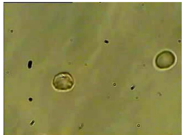
Video 4 Trapping of a flowing, malaria-infected red blood cell (PRBC) by an optical trap. The flow of the medium leads to considerably less elongation of the cell, compared to a healthy cell, due to its enhanced rigidity that accompanies Plasmodium infection. (QuickTime, 831 kb). [URL: http://dx.doi.org/10.1117/1.3037342.4 ].
